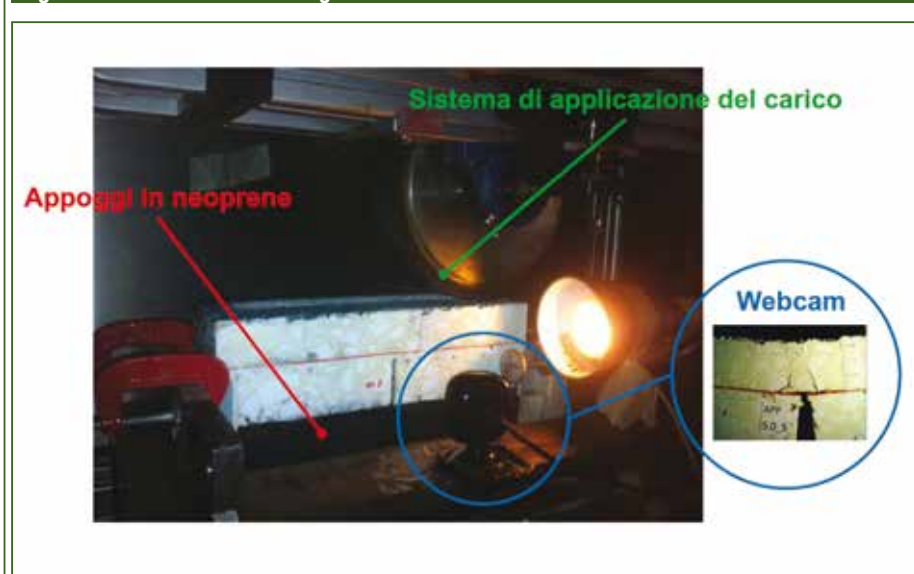
Figura 5. Anti-Reflective Cracking Test
